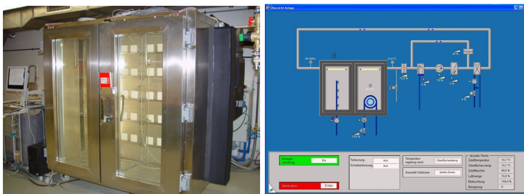
Figure 2: Photograph of the accelerated weathering chamber during operation (left) and a screenshot of the monitoring program (right).
